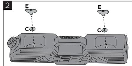
**On the other side, fit the washers (C) and lose with the wing nuts (E) loosely, so as to be able to adjust the stroke and angle of the attachments.**
