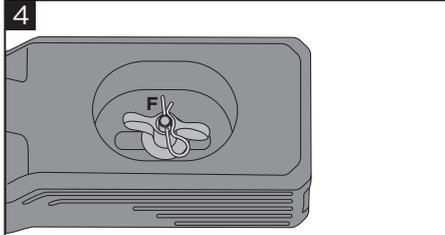
**Close the wing nuts (E) and fix the cotter pin (F).**
