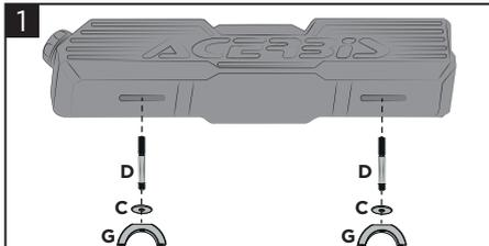
**Fit the connections (G), the washers (C) and the pins (D) on the tank as shown in the figure and tighten completely.**
