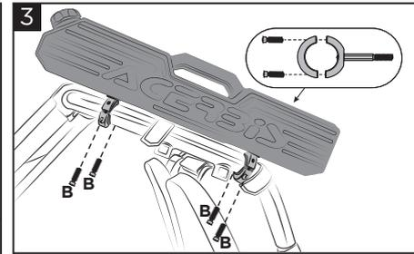
**Position the tank on the vollbar/bullbar and mount using the attachments (H) and the screws (B).**
